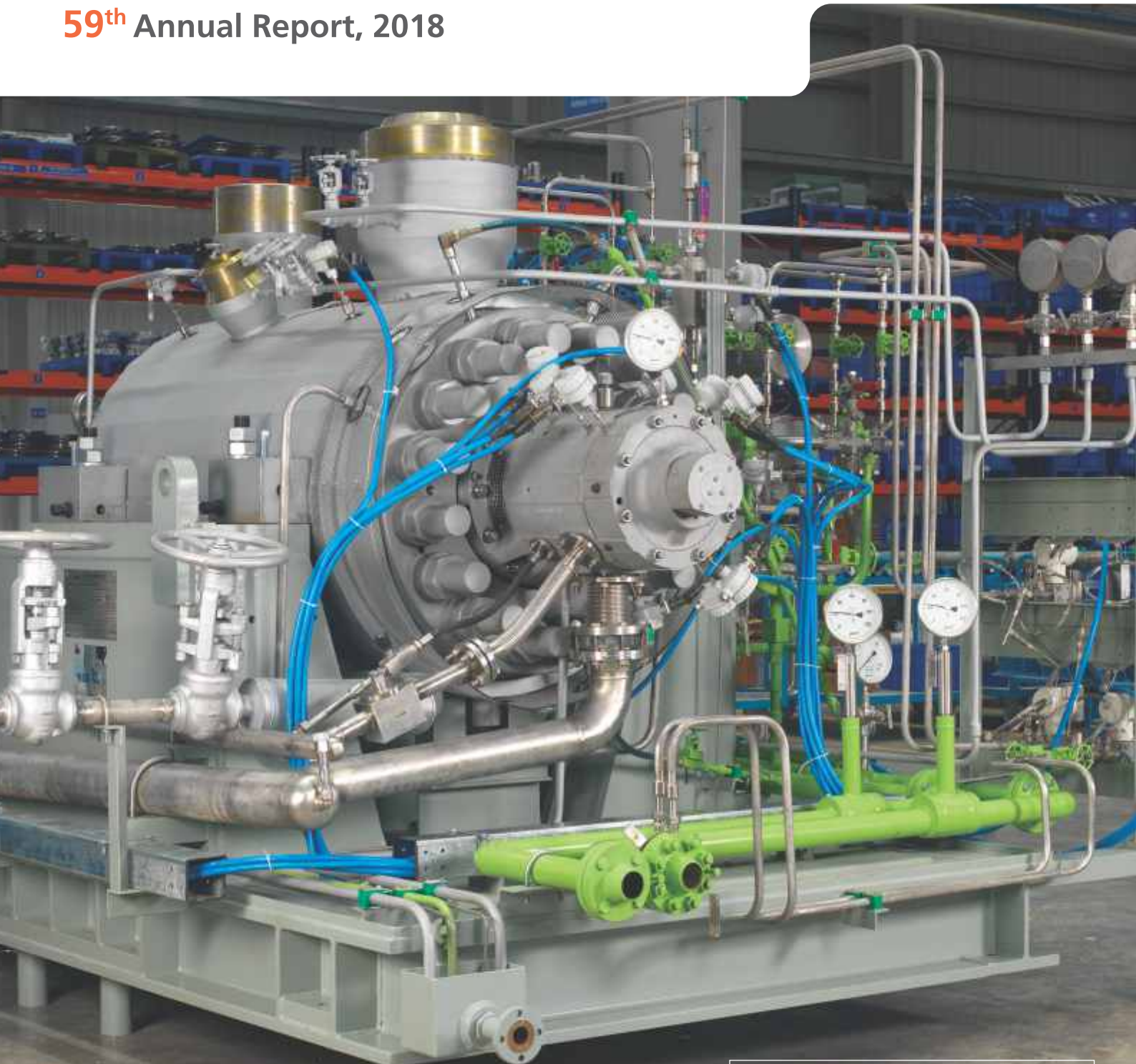
CHTD 6 Pump at Energy Pumps Division
