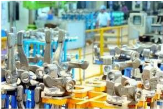
First of its kind Twin Spindle Machines for Front Axle Beam Machining, with shortest cycle times
