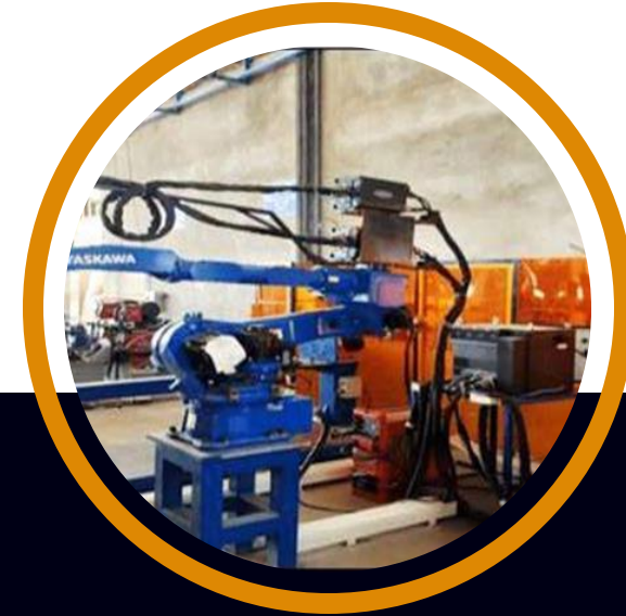
Robotic Twin Torch Welding
