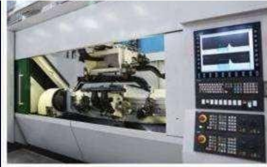
First of its kind Twin Spindle Machines for Front Axle Beam Machining, with shortest cycle times
