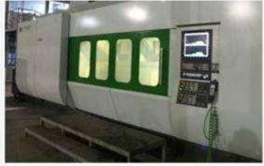
First of its kind Twin Spindle Machines for Front Axle Beam Machining, with shortest cycle times
