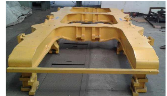
Flexi Curve Loco Bogie- Mozambique
