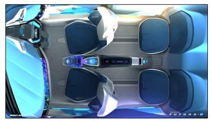
CONCEPT FUTURO-e features flexible swivel travel seats and console which give occupants an unparalleled comfort and freedom to engage freely with infotainment features.
