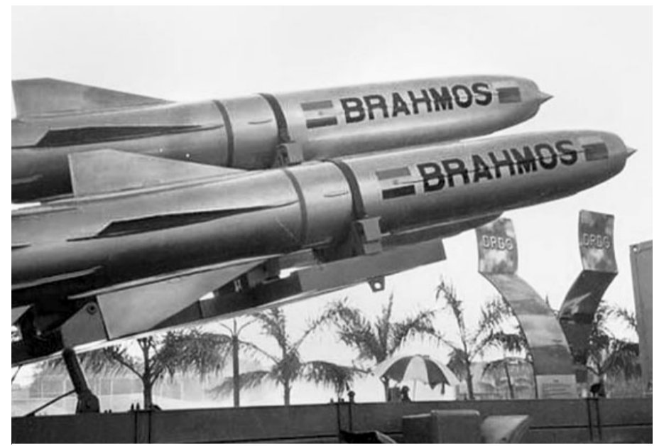
The BrahMos is regarded as one of the world's premier cruise missiles, with its supersonic speed of 2.8 Mach (almost 3,000 kmph) making it extremely difficult for enemy fighters to intercept and shoot down
