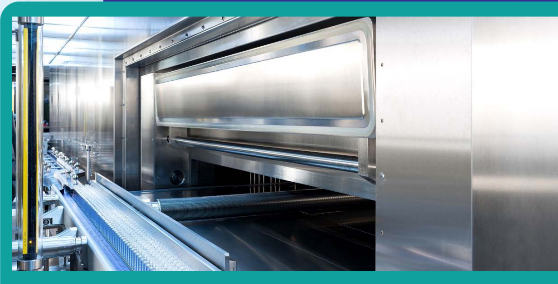
Lyophilizer with Automatic loading and unloading system
