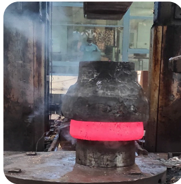
Hot deformation of conical forging
