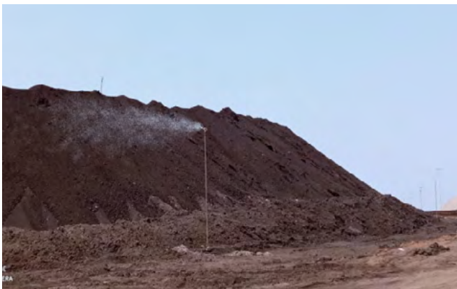
Spray Guns in Bunker Area
