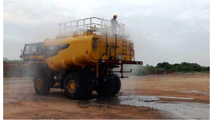
BEML Made Mist/Fog and rain gun water sprinkler deployed for arresting Fugitive emission
