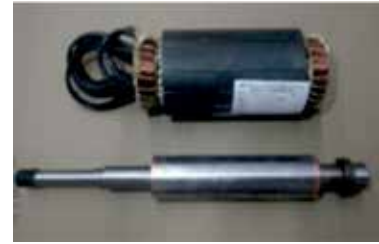
KU6 Oil Filled Wound Stator and Rotor
