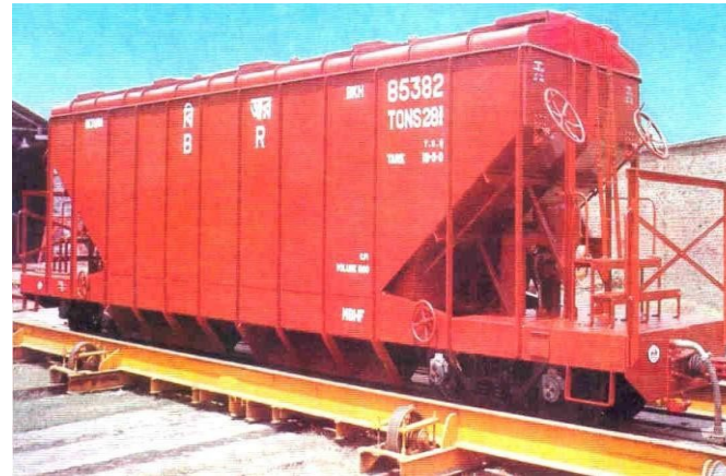
Covered side discharge hopper car for Bangladesh railway
