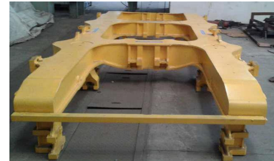
Flexi Curve Loco Bogie- Mozambique
