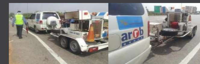
Falling Weight Deflectometer (FWD) Analysis Identification of Weak Spots via Non-destructive Tests
