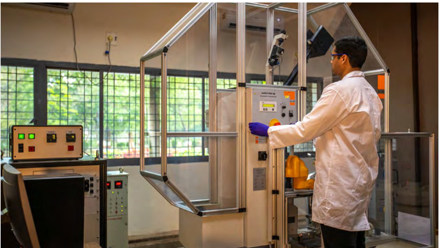
Impact Testing using Fully Automated Robotized Impact Test System at BHEL Corporate R&D, Hyderabad
