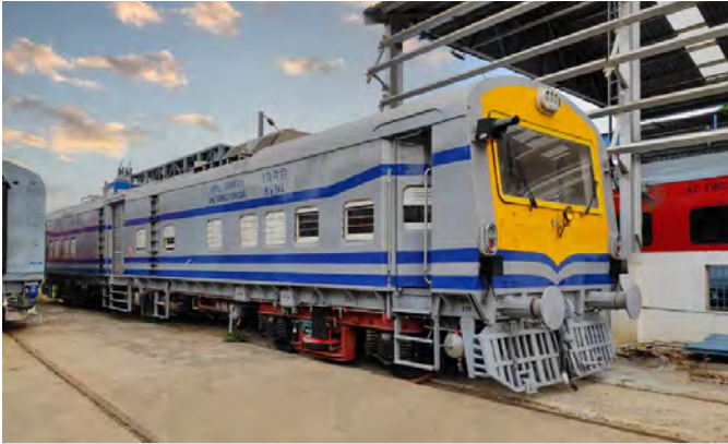
Diesel Electric Tower Car
