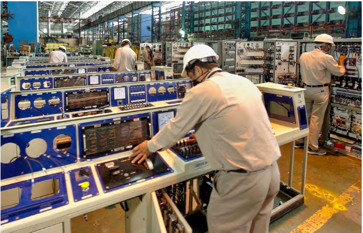
Control System Manufacturing at Switchgear Division (SCR), BHEL Bhopal for DETC (Diesel Electric Tower Car)
