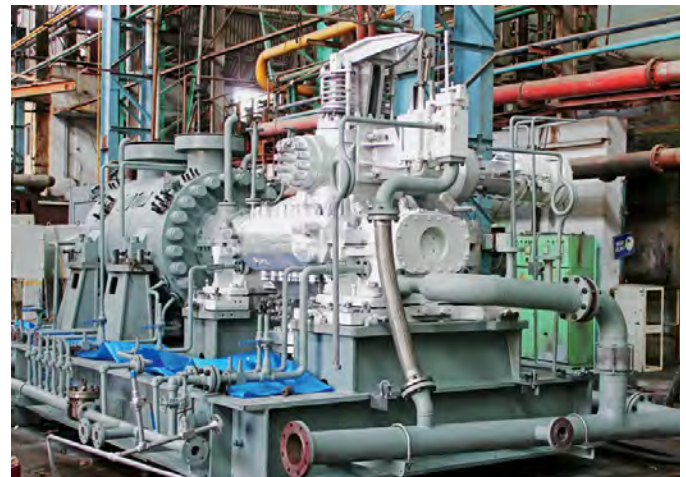
Centrifugal compressor manufactured by BHEL
