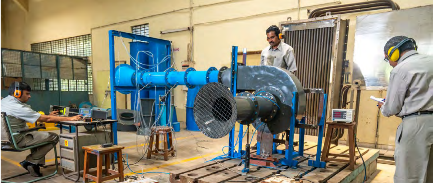
Radial Fan test track at Centre of Excellence for Heat Transfer and Fluid Flow at Corporate R&D, BHEL Hyderabad
