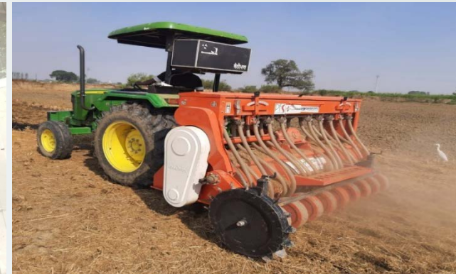
Ongoing project of Crop Residue Management in Ludhiana & Patiala. A Happy Seeder in action.
