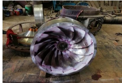
FRANCIS RUNNER ASSEMBLY UNDERGOING NDT TESTING FOR UPPER KALLAR HYDRO PROJECT, KERALA
