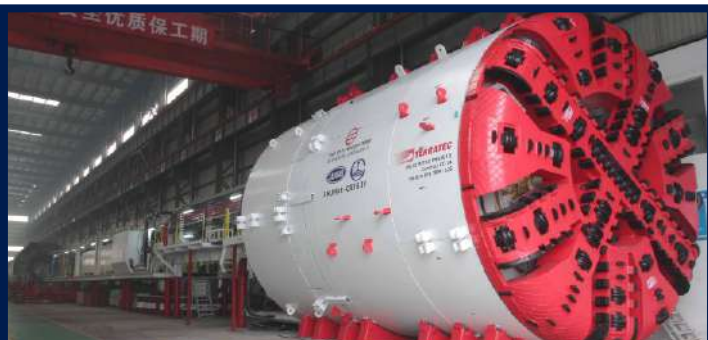
Tunnel Boring Machine (TBM)
