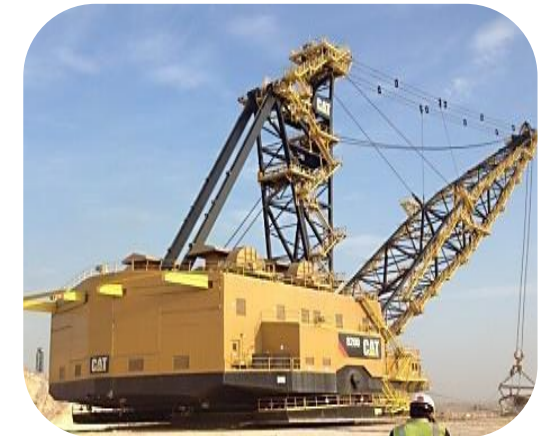
Reliance - Sasan Coal Mine (one of the world's largest dragline - Caterpillar) - Hoist & drag rope
