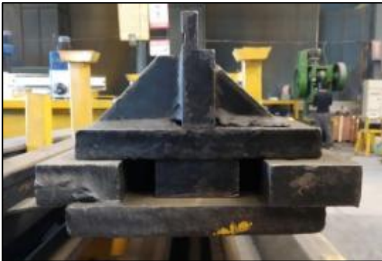
Company Owned Die Punches For Corrugation
