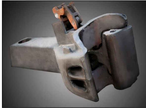
Passenger Coupler with balance Draft Gear
