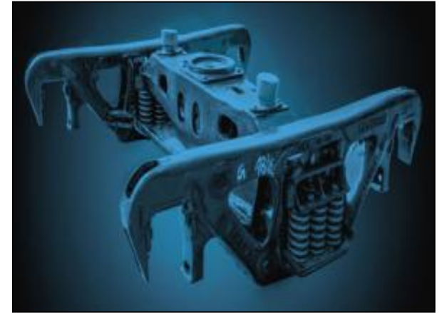
Alloy Steel Cast Bogie
