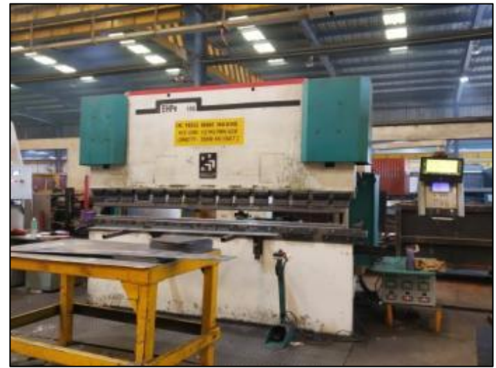
3 Mtr Bed Brake press to handle corrugation
