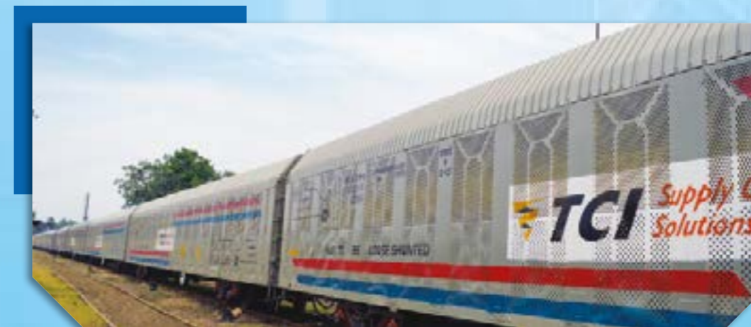
Autocar Carrying wagon rake (BCACBM), manufactured by Texrail and supplied by Texrail Touax JV
