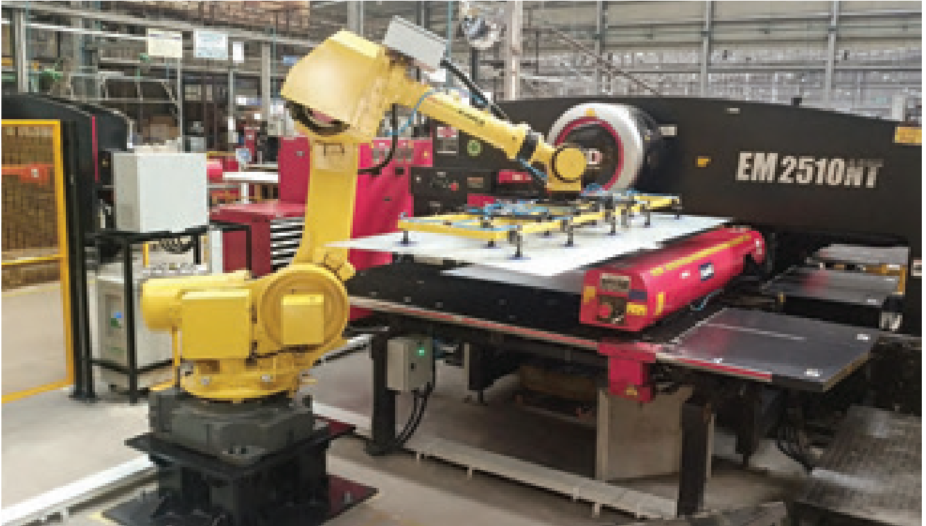
This robot at Wada Plant has been installed on the Amada Turret punching machine for sheet metal 'Pick & Place' process. It is Fanuc make, with a 165kg payload capacity. The robot has eliminated human fatigue and increased machine utilisation by 15%
