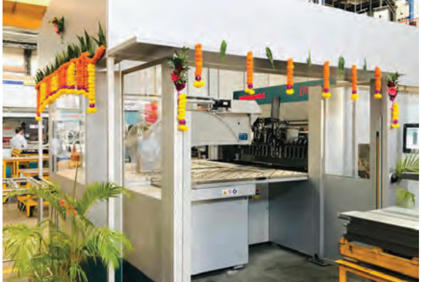
The new Salvagnini Px installation at Dadra Plant efficiently bends sheet metal for product chassis, thereby increasing the capacity of the Plant
