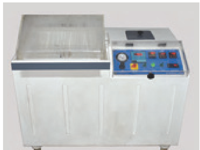
The salt spray test chamber, where components such as nuts and bolts, sheet metal and electronic PCBs are tested
