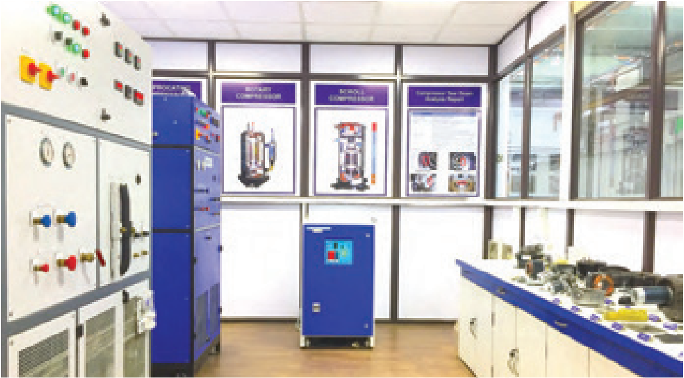
Compressor Lab comprising of two Compressor Test Rigs and Cut Sections of Tested Compressors at Blue Star's R&D facility in Thane
