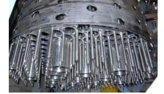
Control Plug for Reactor
