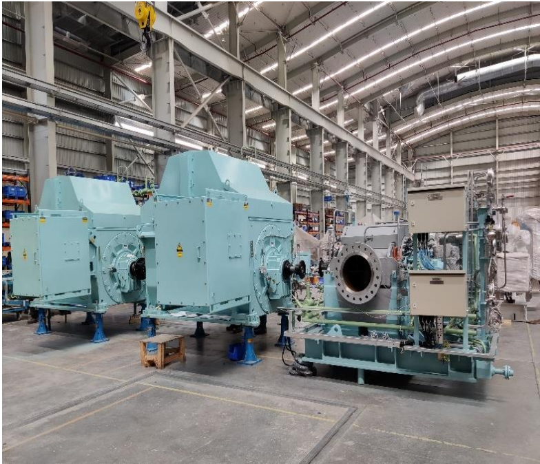
Boiler feed pump for supercritical power plant 660 MW End client - Vietnam power corp.
