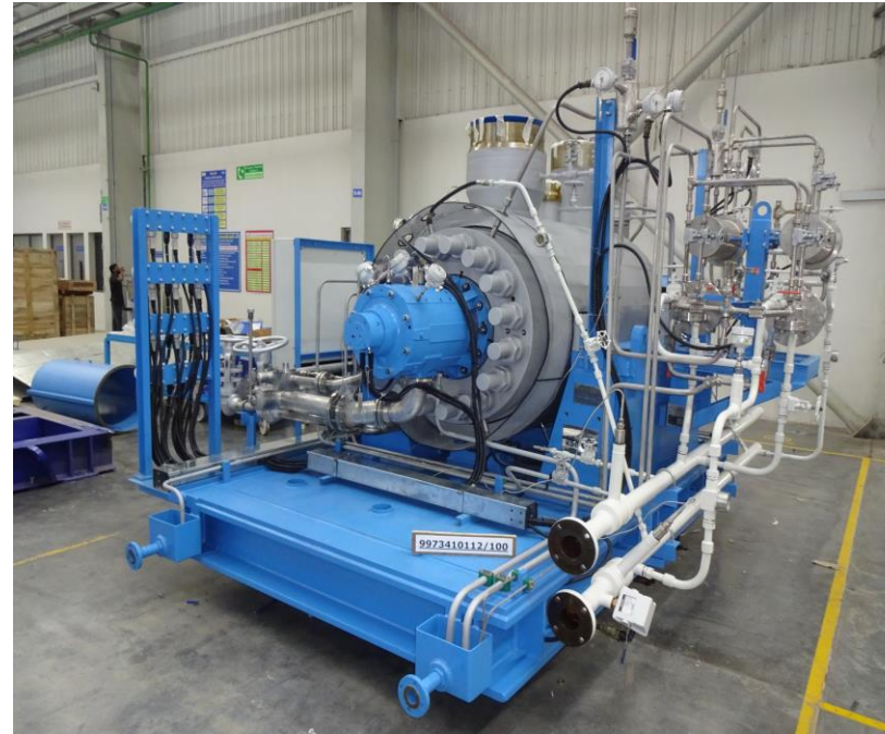
Boiler feed pump for supercritical power plant 800 MW End client - NTPC
