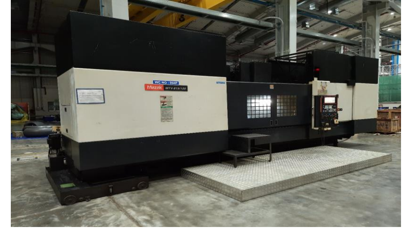
VMC, For drilling & keyway milling operations. Longest shaft of 3.2 meter holding
