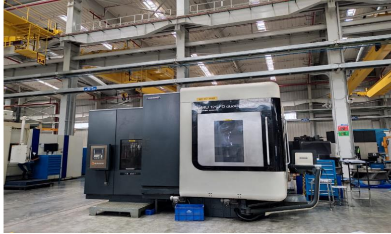
VMC , 5 Axis multitasking machine Having Features of turning & Milling
