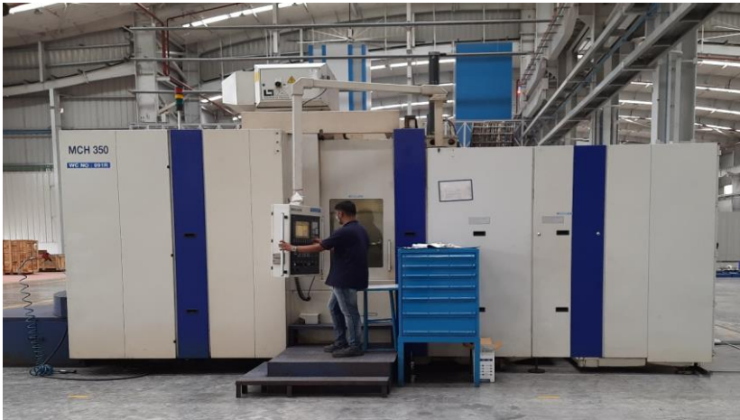
HMC For Flange machining & Feet Machining
