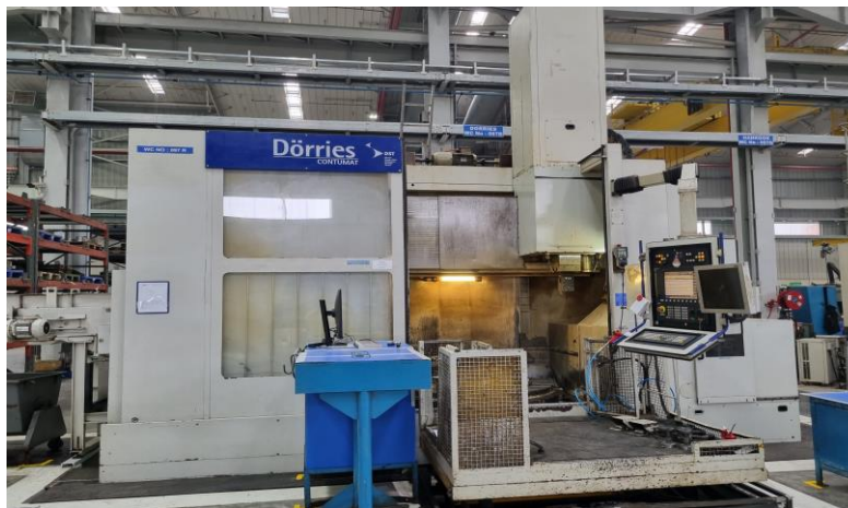
VTL For Barrel & distributor casing Machining.
