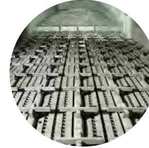
First in India to install Cross bar cooler to reduce specific fuel consumption
