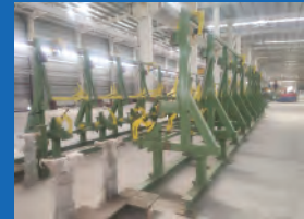
Sidewall & Carline Intergration Fixture
