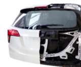
Plastic Tail Gate Modules (Lighter in weight)
