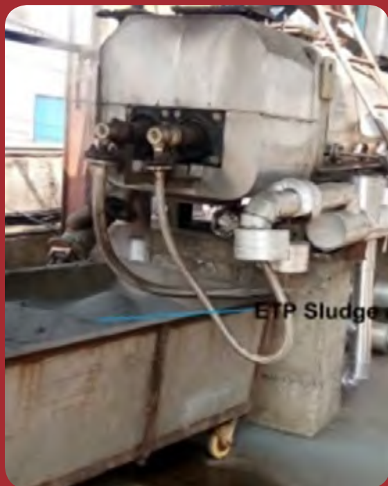
ETP Paddle dryer with dry sludge
