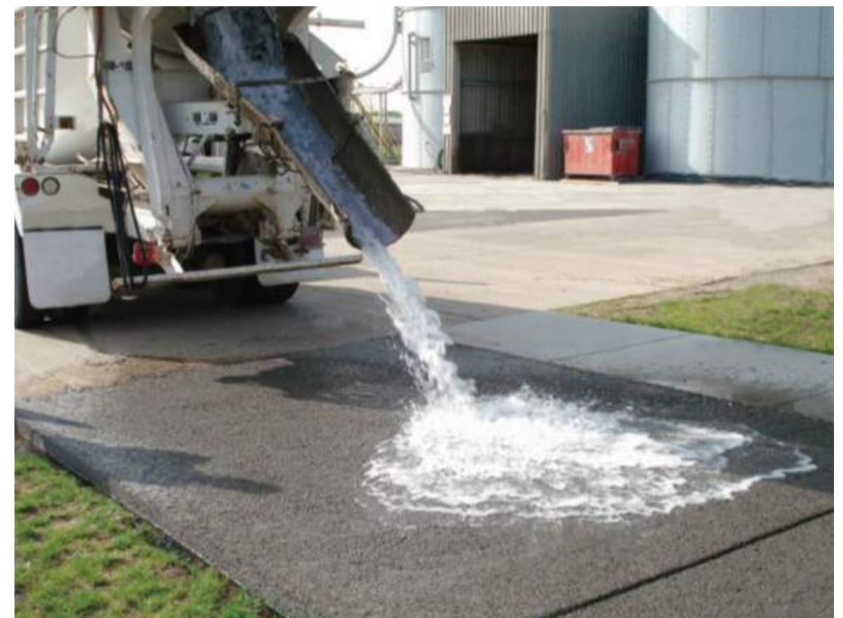
Perviouscrete concrete prevents water-logging and keeps the surface dry.
