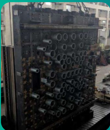
Calandria Vault Top Hatch Cover Beam
