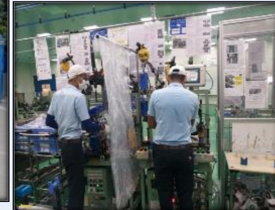
Separation curtain between the operators
