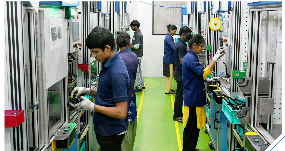
Assembly of Disc Brake Systems in our new E-71 Plant at Waluj, Aurangabad
