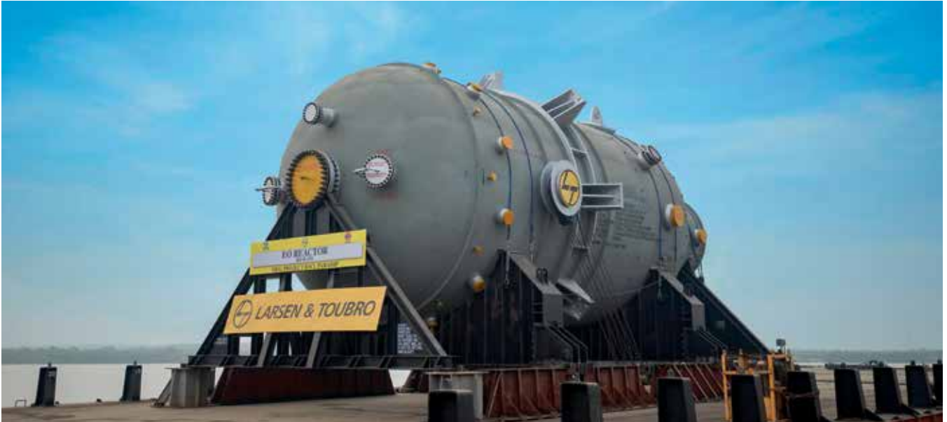
Ethylene Oxide Reactor weighing 1157 MT for IOCL's Paradip Refinery
