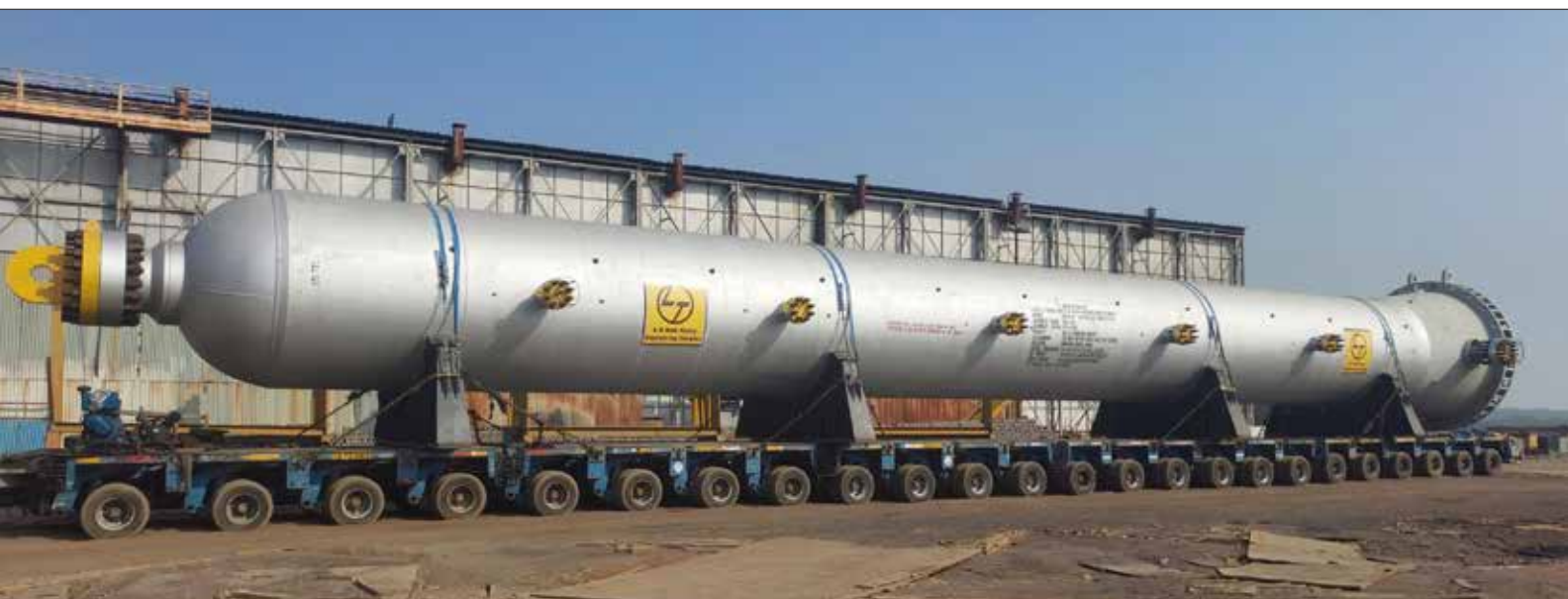
OHCU Reactor for IOCL Barauni BR-9 Expansion Project, Bihar
