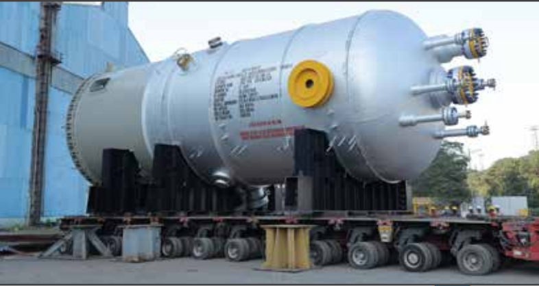
PTA Crystalliser for a Petrochemical Company in Turkey
