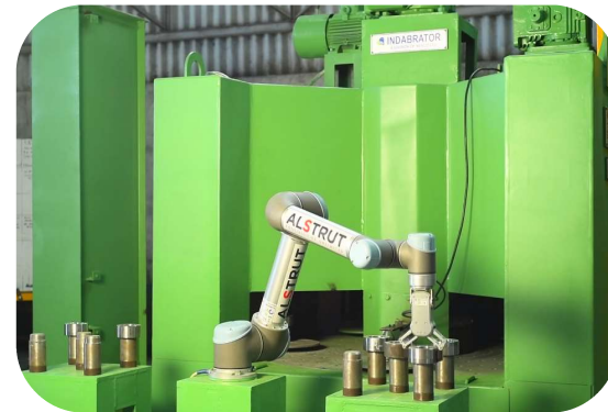
Shot Peening machine with Robotic Pick & Place
