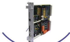
Railway Embedded Controller
