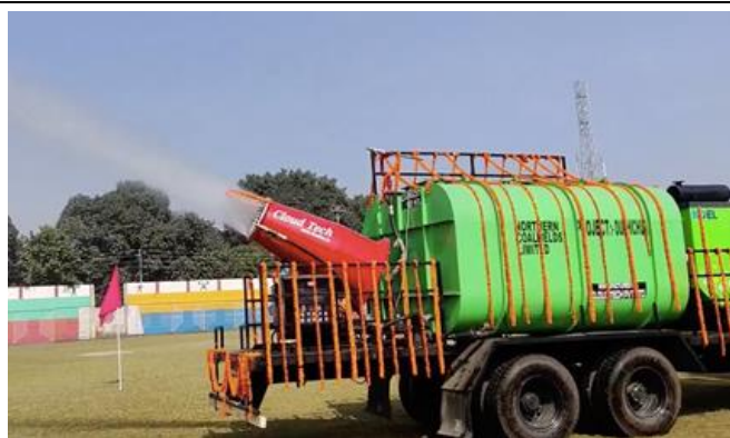
Fig. 49 - Coal India Limited has commissioned two mist cannon sprays in Northern Coalfields Ltd. The mist cannon spray is mounted on trucks to suppress the dust in its mining operations. With a tank capacity of 12,000 liters, the mist cannon spray rapidly suppresses dust before it can disperse during mining operations. It has a mist spray throw of 90-100 meters and an oscillation of 360 degrees
