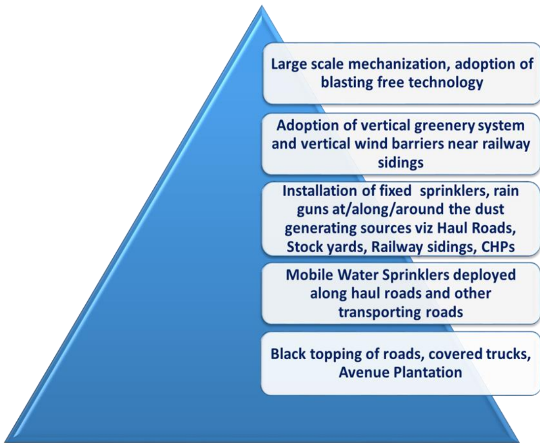
Fig. 47 - Air Pollution Control Measures
