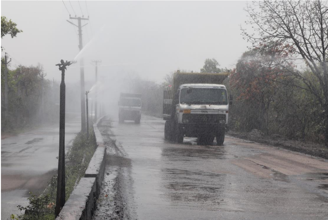
Fig. 45 - Water sprinkling in Coal Transport Roadways
