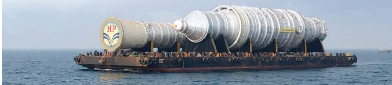
On Voyage - CDU & VDU Columns for Visakh Refinery Modernisation Project
