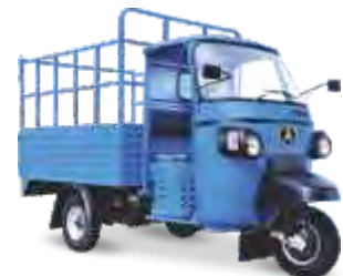
FRONT ENGINE HIGH DECK 500 KG PAYLOAD CAPACITY
