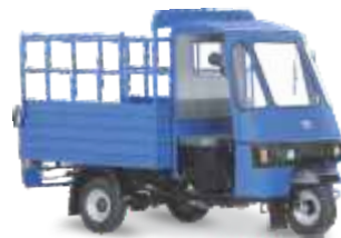
FRONT ENGINE HIGH DECK 500 KG PAYLOAD CAPACITY
