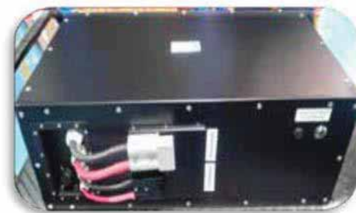
Golf Cart Battery Pack
