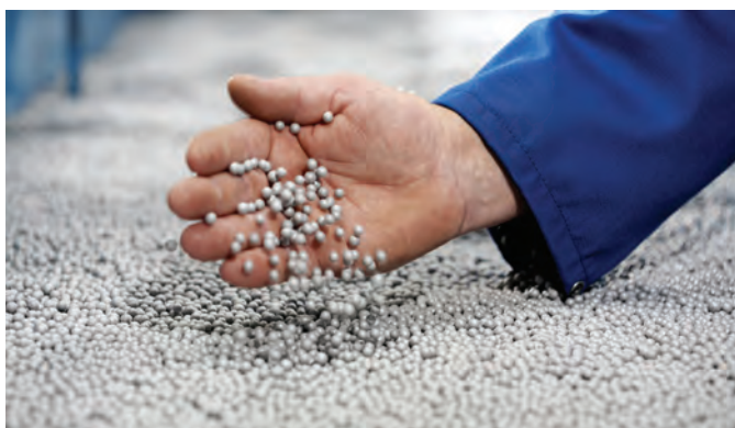
Foamed Neopor® is as light as a feather: the silver-gray beads are formed as a result of the prefoaming process and is an innovative insulating material offered by the Petrochemicals business of your Company for construction industry.
