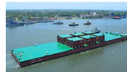
Deck Cargo/ Jacket Launch Barges
