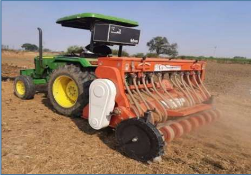
Ongoing project of Crop Residue Management in Ludhiana & Patiala. A Happy Seeder in action.
