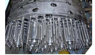
Control Plug for Reactor
