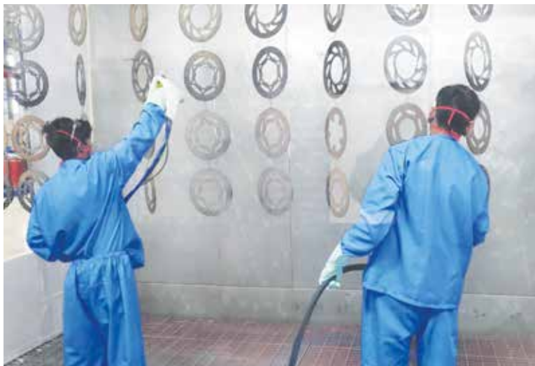
▲ Spray painting of Brake Discs at Waluj, Aurangabad
