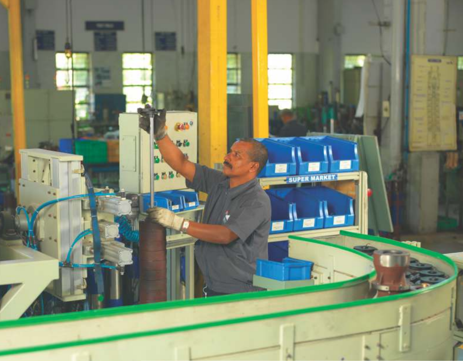
Automation of assembly line of 150 mm submersible pumps at Sinnar plant.
