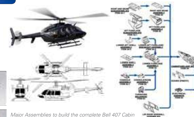
Major Assemblies to build the complete Bell 407 Cabin
