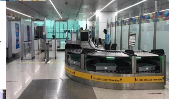
Automatic tray retrieval system at Delhi Airport
