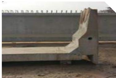
Fabricated Casting Panels and Moulds
