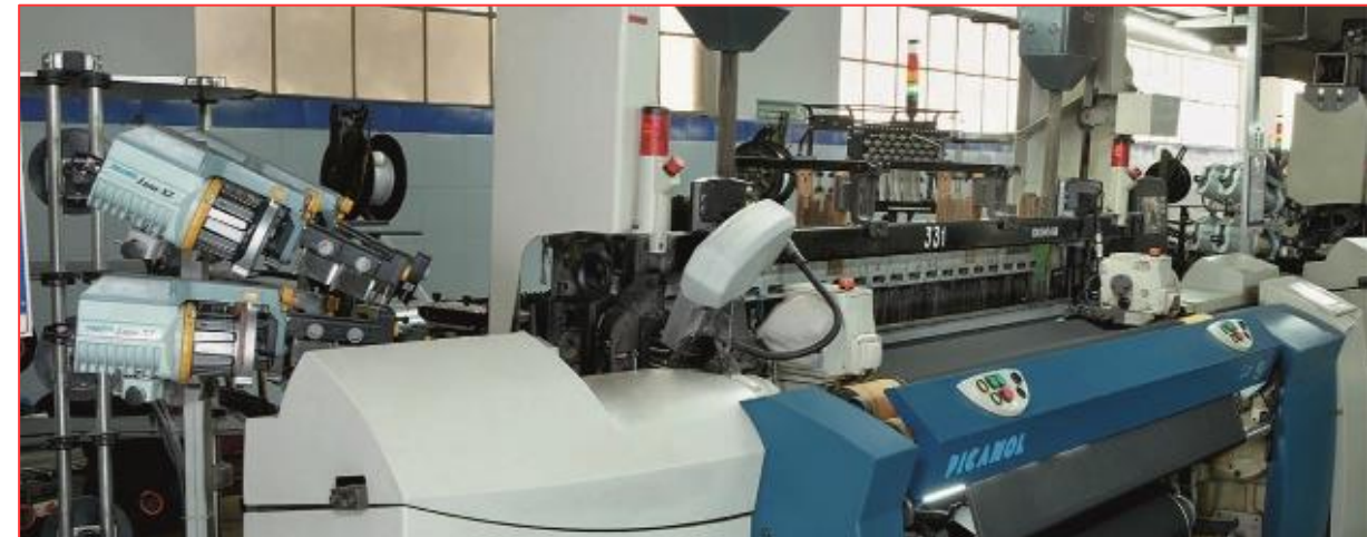
Weaving technology like Rapier: Picanol (Belgium) and Dornier (Germany), Projectile: Sulzer Textile (Switzerland), Airjet: Toyoda (Japan)
