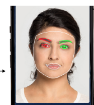
1. Face stillness check across all frames (using relative movement of facial coordinates)
