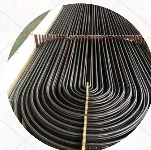
U Bending + Annealing facilities for Heat Exchanger Tubes
