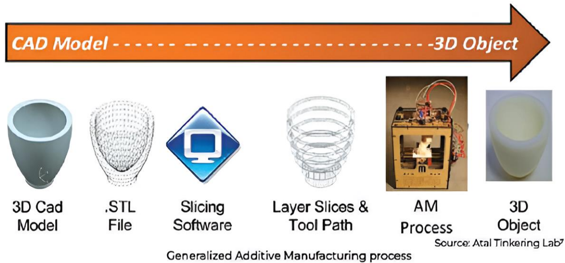
Fig.6 Basic Additive Manufacturing process
